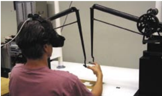
A subject using a visual-haptic virtual reality environment. The subject sees virtual objects rendered in the head-mounted display, and grasps these objects using the force-feedback devices connected to his thumb and index fingers.
