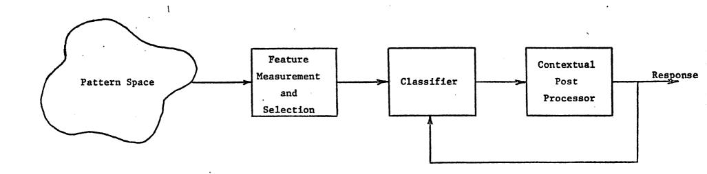
Figure VII.1 Recognition System Utilizing Feedback of Contextual Information: feedback from contextual post processor to classifier indicates the reduced set of alternative characters. Reclassification is performed on the reduced set.
