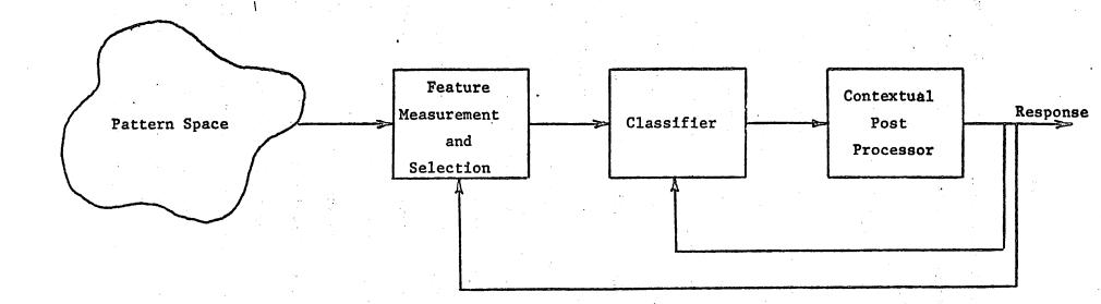
Figure VII.2 Complete Recognition System Utilizing Two Modes of Feedback: feedback from contextual post processor to classifier reduces the number of alternatives when reclassification is indicated; feedback from contextual post processor to feature measurement and selection indicates additional specific measurements to be made.
