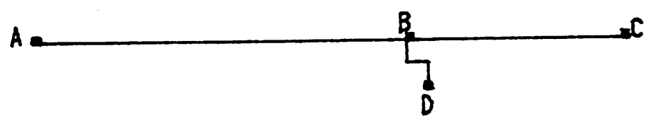
Figure 14. BD should be eliminated as a low-confidence edge. AB and AC should be merged to form AC which, being longer, will be more confident than AB or BC.
