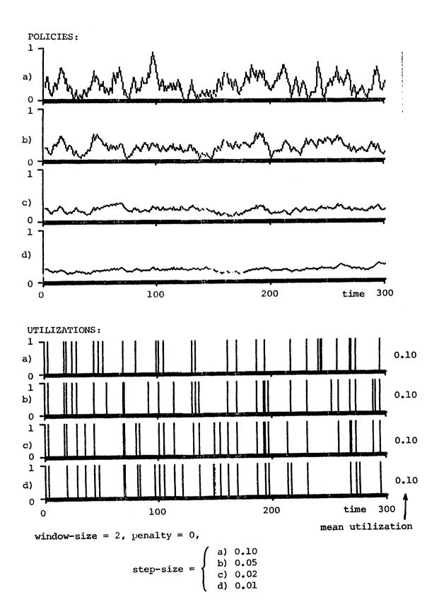
Figure 4: Probabilistic Scheme at Equilibrium with various step-sizes
