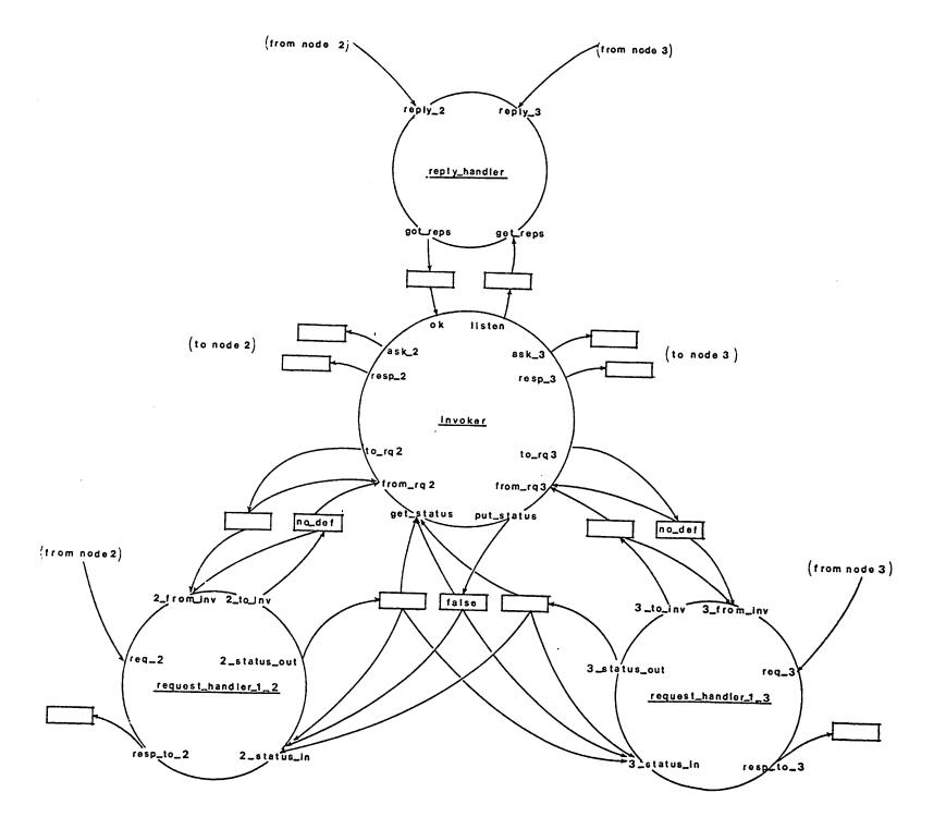
inbound and outbound ports are represented by inbound and outbound arcs, respectively, and links are represented by boxes. This figure also shows the messages that are assumed to be initially available through the communication linkages. A character string, such as "no\_def", inside a link represents an available message, while an empty box indicates that no message currently resides in that link.
