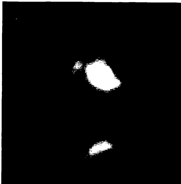
Figure 3.8b: LA-TS imprint of the front of a nickel under 28.9 N load. The WP125 transducer membrane and RB380 cover membrane was used.
