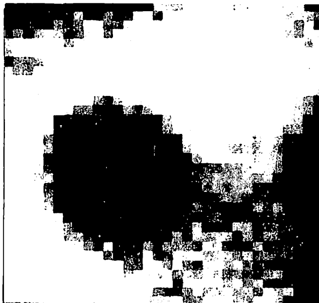
Figure 14: SCREEN1-HARD – Heavy screen contact (square grid)
