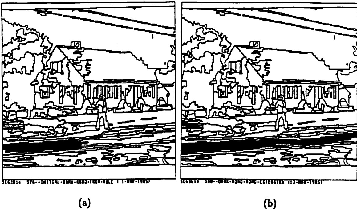
Figure 31. Results for Road Interpretation Strategy (a) The initial region and (b) the extension produced by the road interpretation strategy.
