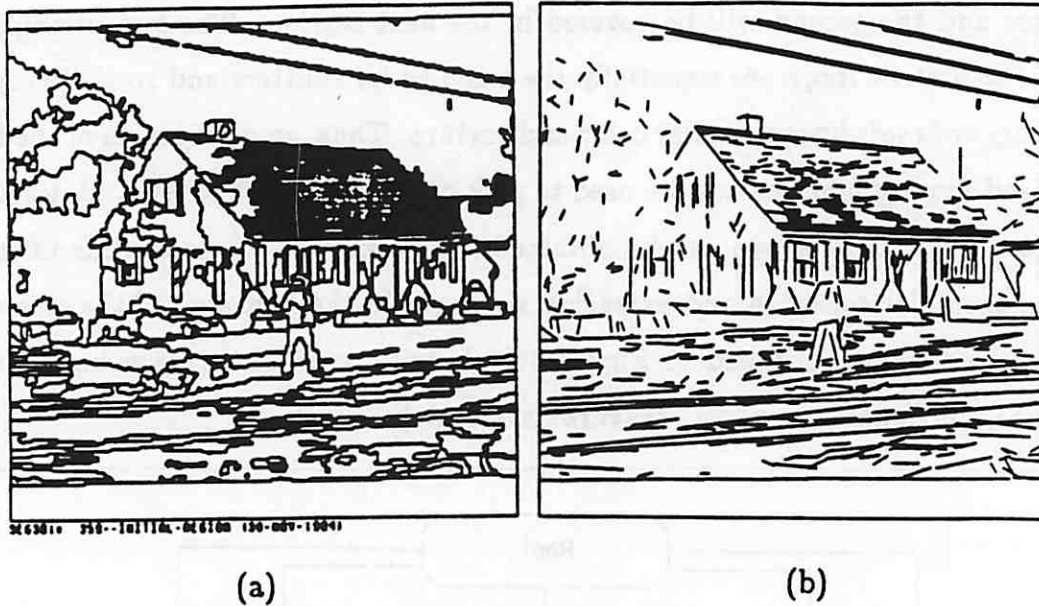
Figure 33. Initial Roof Region and Line Data (a) Shows the region selected as the roof exemplar and (b) the lines from the image data base.
