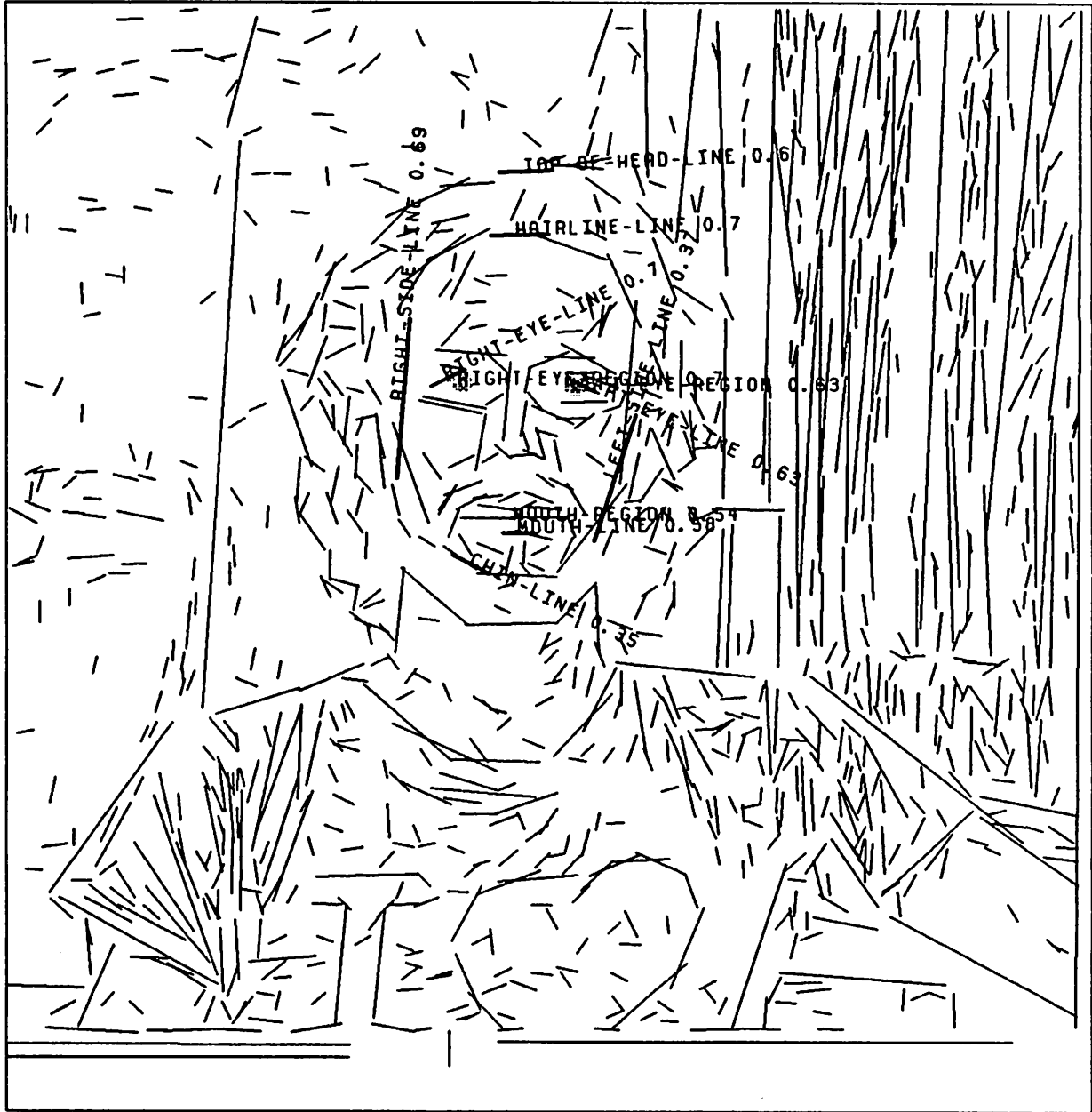
Figure 21: "Les" model against "Les" image 3: Best matches for each face part after four iterations of relaxation matching.
