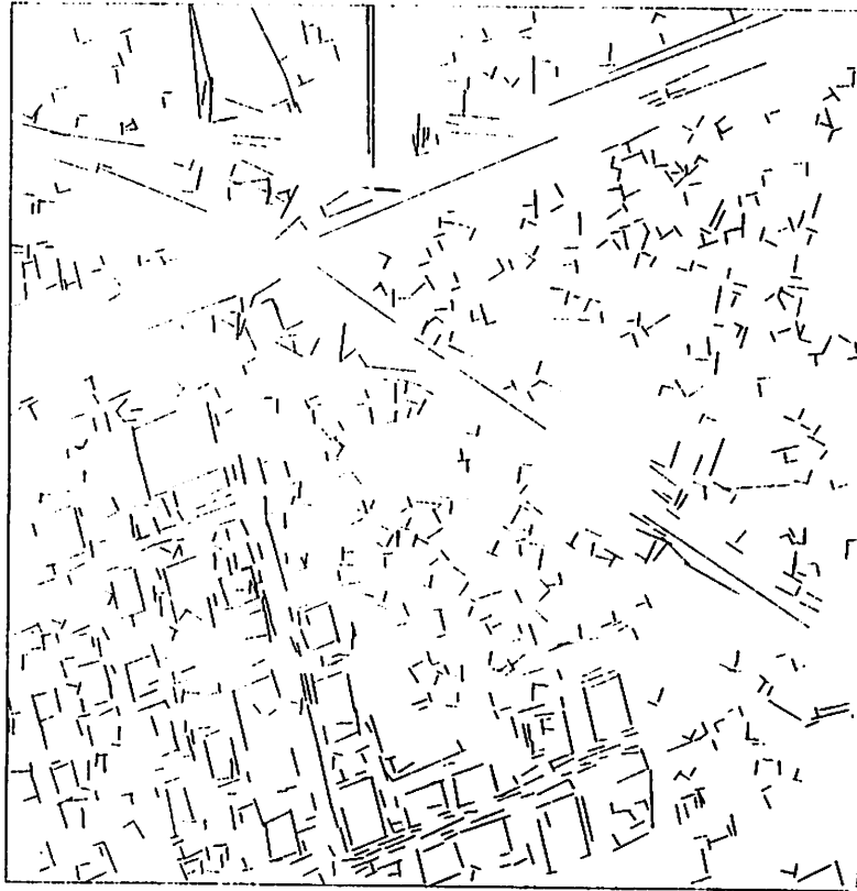
Figure 17: Lines Belonging to Spatially Proximate Orthogonal Pairs for the Aerial Photograph.
