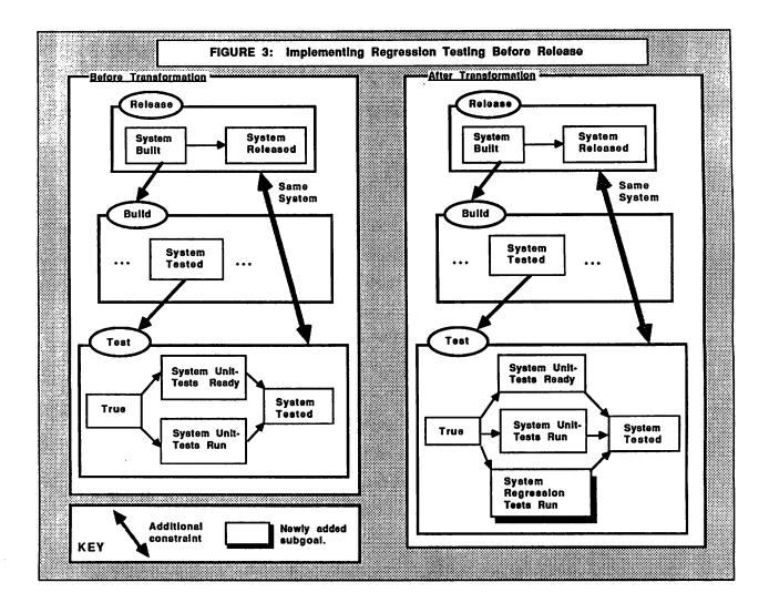
Assuming the *test* operator of Figure 1, the effect of the transformation is to add an additional subgoal to run the regression test cases. The formula defining the new subgoal is supplied explicitly in the transformation -- it need not have appeared previously in the plan network. Only the one operator instance is modified; the basic operator definition for *test* is unchanged. The results of applying this transformation are shown as the AFTER case in Figure 3.
