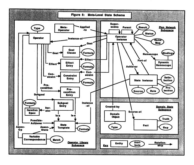
states and status (pending, achieved, protected...). Also associated with operator instances are the dynamic name scopes and variable binding information needed to evaluate operator formulas. The domain state represents the truth value of all domain predicates. Additional predicates cross subspace boundaries, relating operator instances back to their definitions, and operator instances to the domain predicates they affected.
