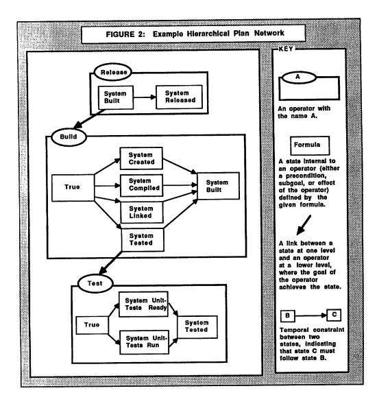
instantiated operators consist of additional states describing the internals of the operator: preconditions, subgoals, and effects. Arrows within levels show how the achievement of certain states is partially ordered with respect to time (some orderings are specified by the operator definitions and other orderings are imposed to resolve interactions). Orderings are propagated from level to level, but have been omitted to simplify the figure.
