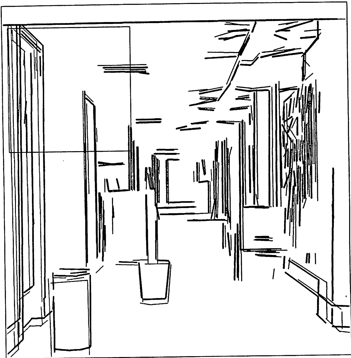
Figure 71: The hallway-scene experiment: The lines extracted by Boldt's algorithm from the two input frames. The thick lines are those from the first frame, while the thin lines are from the second input frame. The area within the rectangular box in the upper left corner of the image will be more closely examined in the next two figures.
