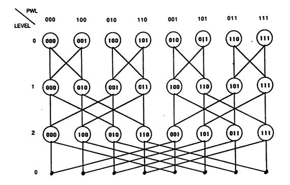
Figure 3. Illustrating  $\Delta(3;2)$  as a coset graph of  $\tilde{B}(3;2)$ .
