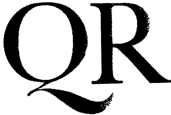
Figure 23. Bitmaps produced by the Ikarus system from the outlines in Figure 22.
