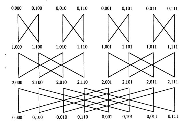
Figure 2. The order-3 butterfly graph  $\mathcal{B}(3)$  with level 0 replicated to aid visualization.
