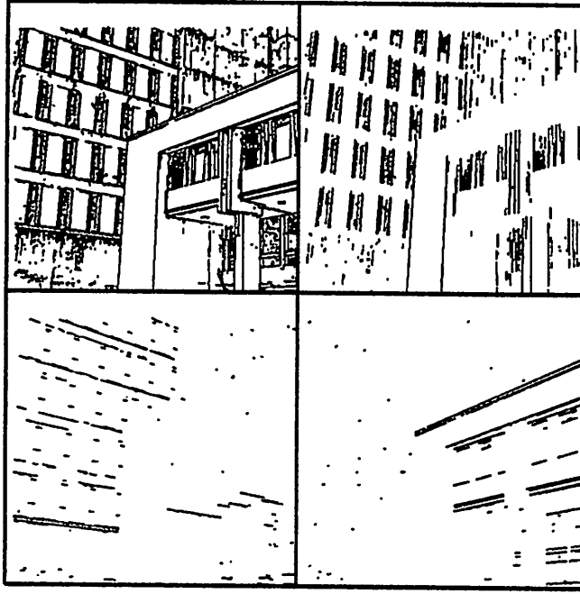
Figure 6: Straight line segments from an outdoor building scene (upper left), and three clusters of converging lines found using Barnard's histogram method [3].
