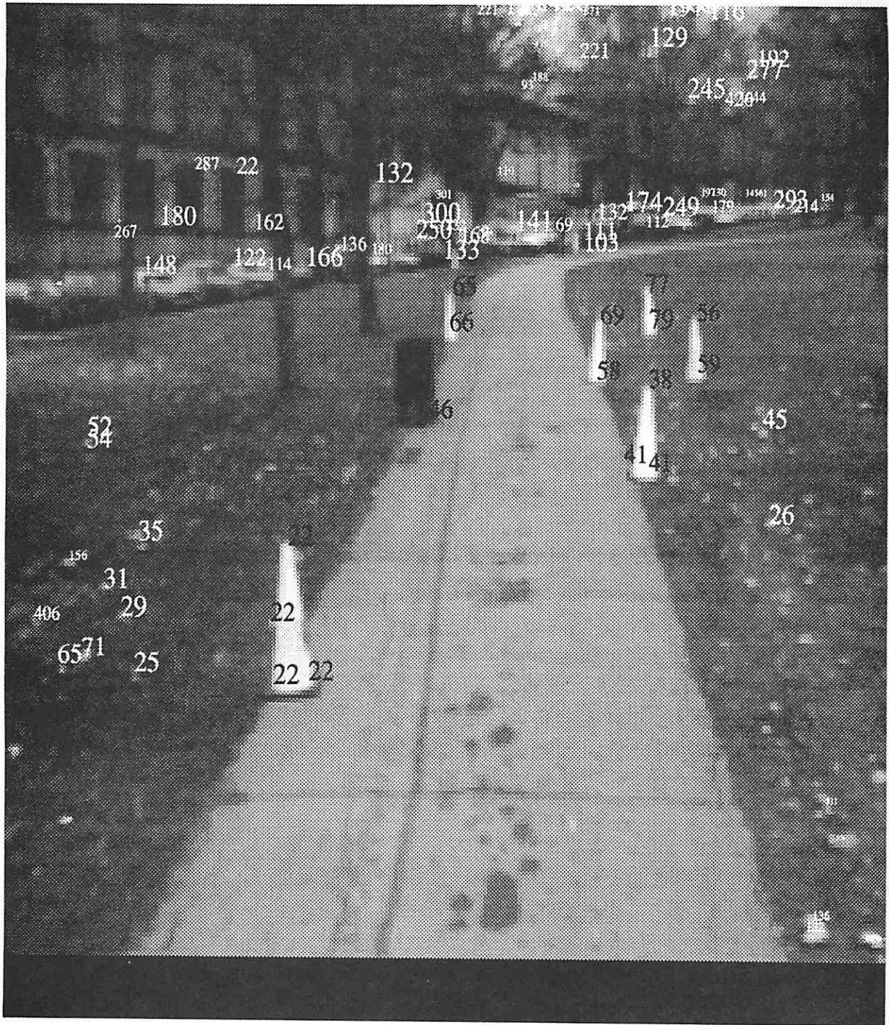
Figure 8: Depths found at all Moravec points in the first frame. A few points have been deleted or shifted slightly for clarity. The better the reliability ( \zeta ) of the depth values the larger the size of the font in which the depth is typed. Ground truths are known for the depths typed in black.
