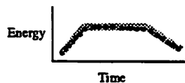
Figure 8: MICROSTREAM LEVEL: The fourth evidence abstraction level contains microstream hypotheses supported by one contour or a sequence of contours in time. Each microstream has an energy pattern consisting of an attack region (signal onset – increasing energy), a steady region, and a decay region (signal fadeout – decreasing energy).
