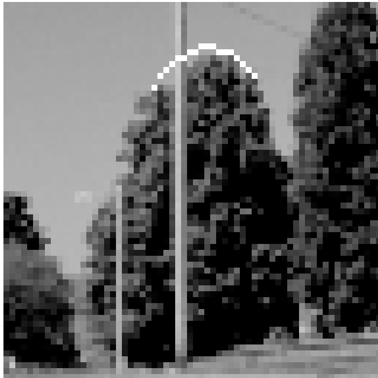
Figure 6.3: Representing the 2D projection of a trees as a parabola in the image. This figure shows a piece of the image in Figure 6.2, including the landmark tree, with a parabola hypothesis representing the location of the tree.
