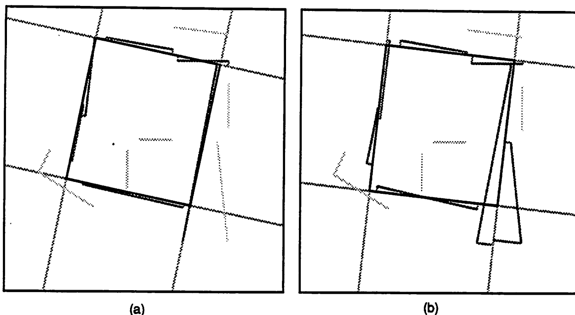
Figure 3.7 Illustrating how perpendicular error is used to measure fit. The error is indicated by lines drawn from endpoints of data segments to extended model lines. Observe how in (b) the addition of one 'incorrect' pairing changes the model's pose.
