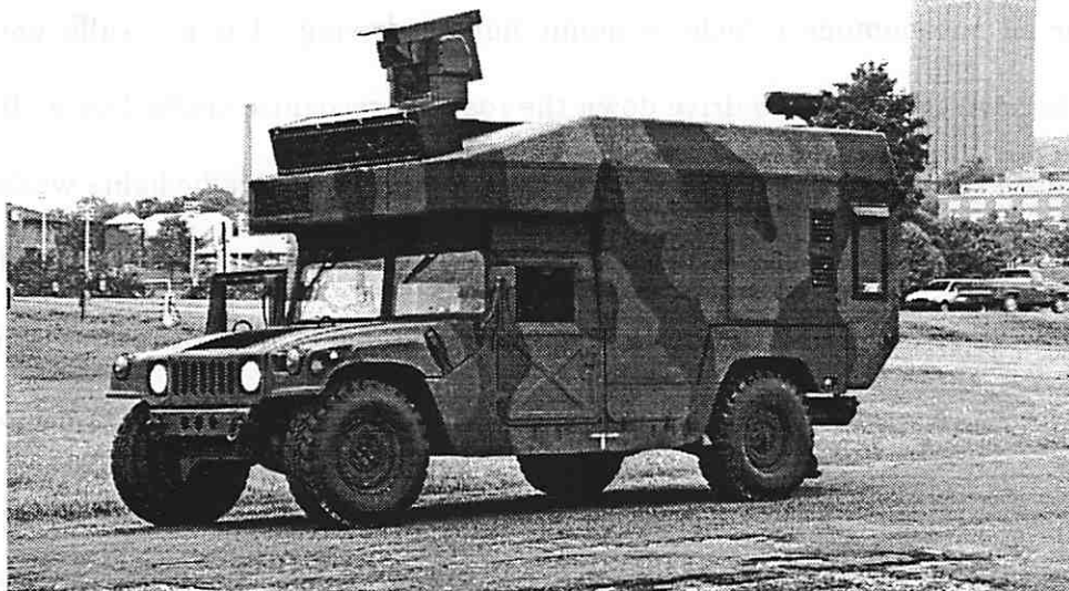
Figure 1: The Mobile Perception Laboratory, built on a modified HMMWV chassis, has computer controlled steering, throttle, and brakes, a complete research laboratory on the back.
