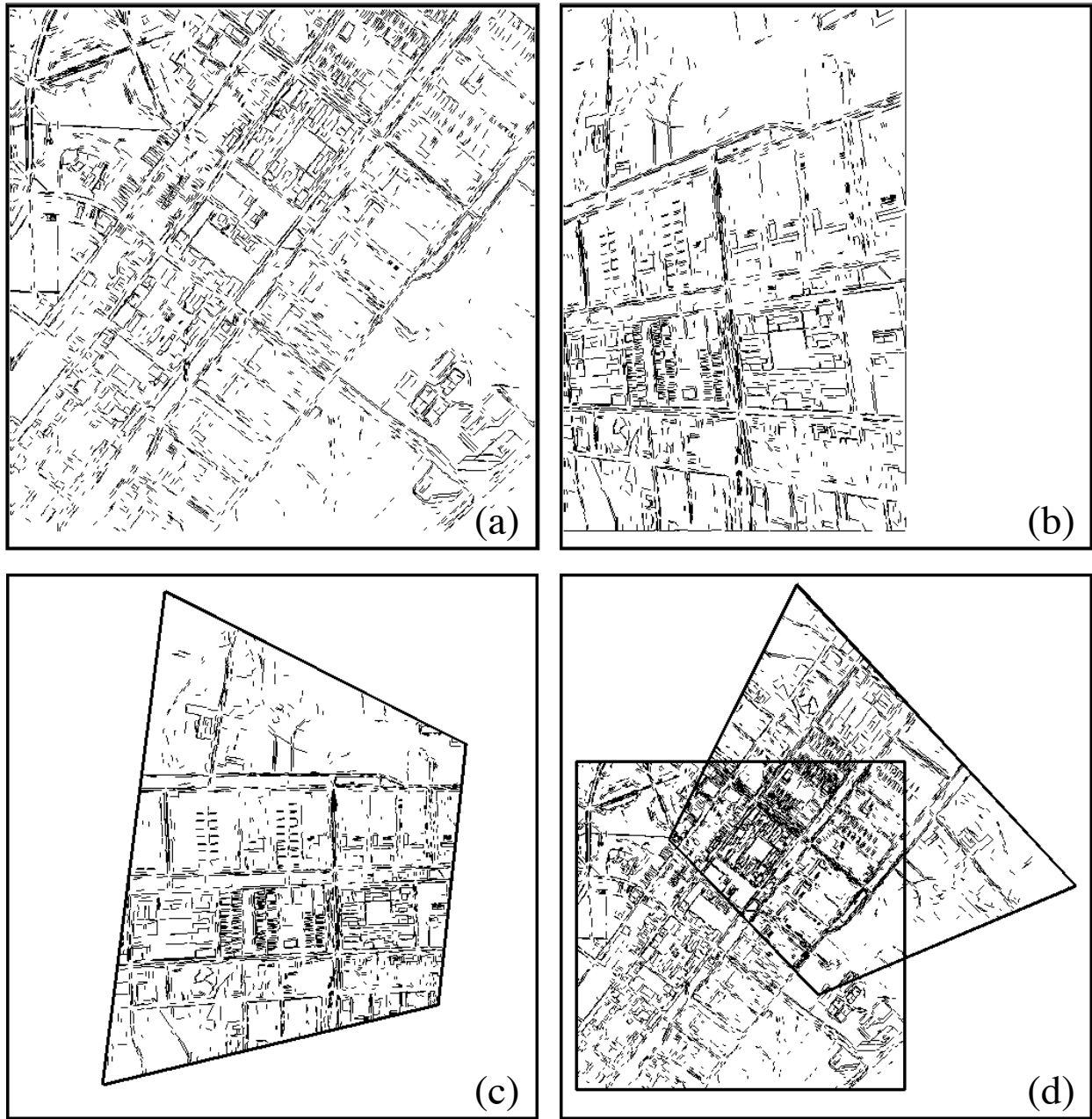
Figure 2: Image-to-image matching example on an aerial image: (a) image lines from nadir view, (b) image lines from oblique view, (c) rectified oblique view, (d) registration of nadir view with rectified oblique view.
