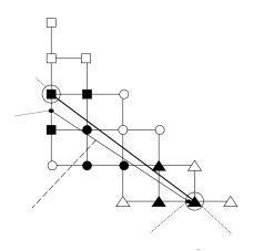
Figure 6: The final line, showing the line from the least squares fit with integer and floating point endpoints.
