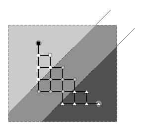
Figure 4: Split of support region into three parts. The black pixel is the arbitrarily chose pixel, which determines the slope of line l1 and l2. The square pixels lie in the light gray area, the circles in the medium gray area, and the triangles in the dark shaded regions.
