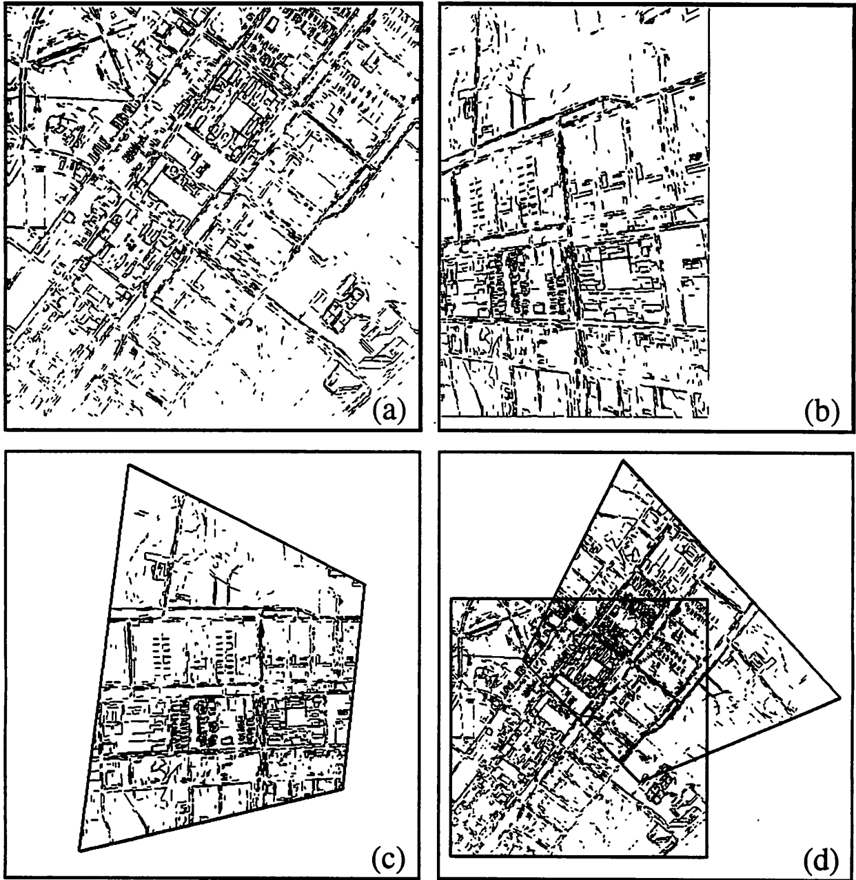
Figure 13: Image-to-image matching example on an aerial image: (a) image lines from nadir view, (b) image lines from oblique view, (c) rectified oblique view, (d) registration of nadir view with rectified oblique view.
