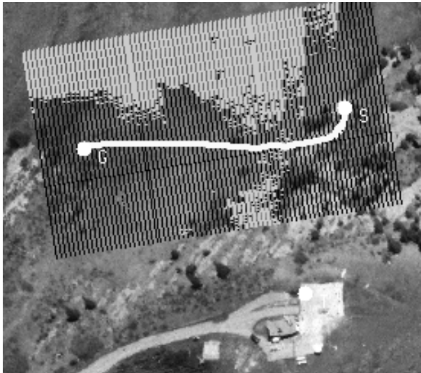
Figure 1: Planning a stealth path from start (S) to a goal (G) on a terrain reconstructed from the DemoB site.
