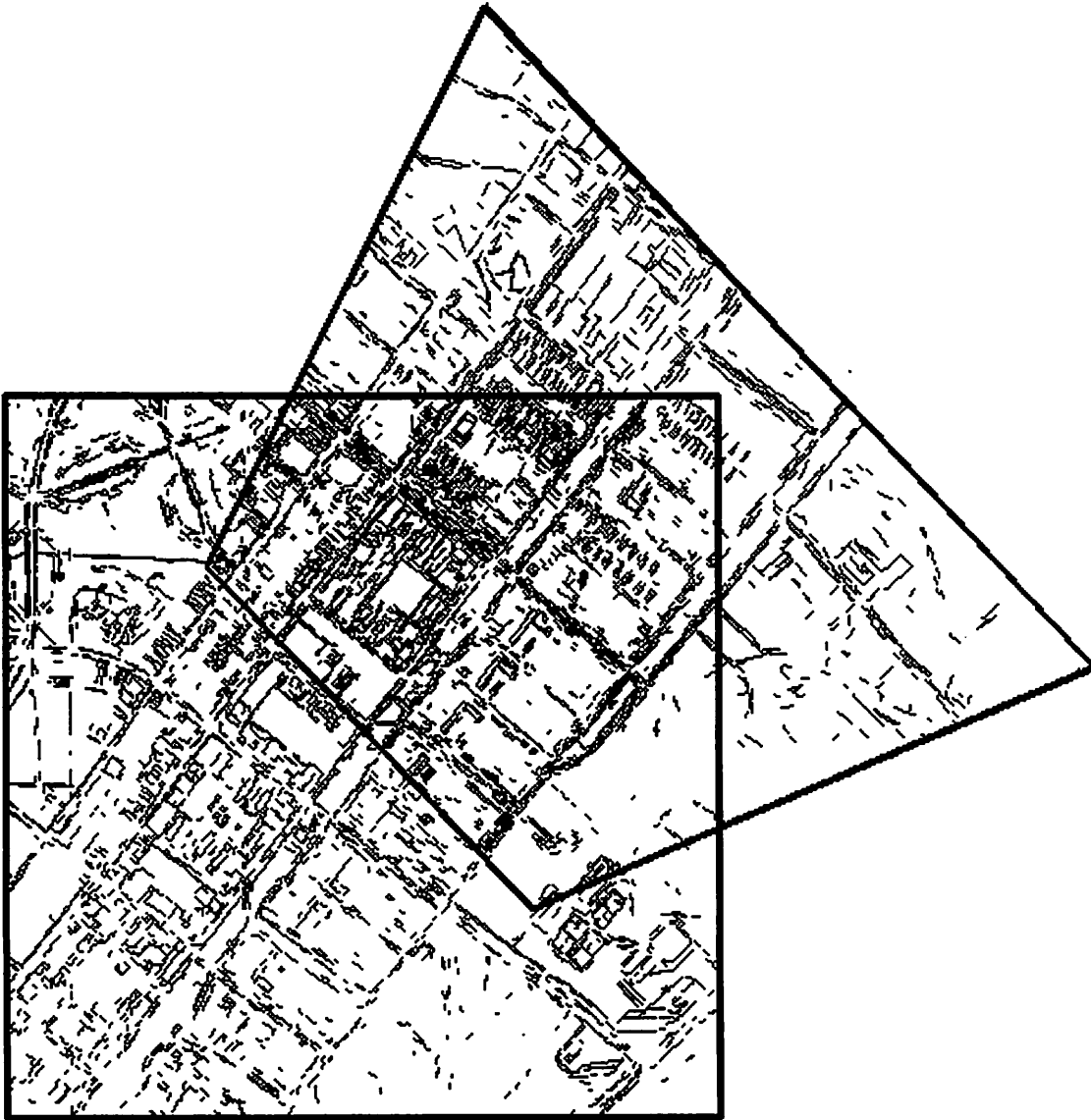
Figure 4.11: A final registered mosaic for the two images in Figure 4.10. Line segments from the oblique view have been projectively unwrapped into the coordinate system of the nadir view.
