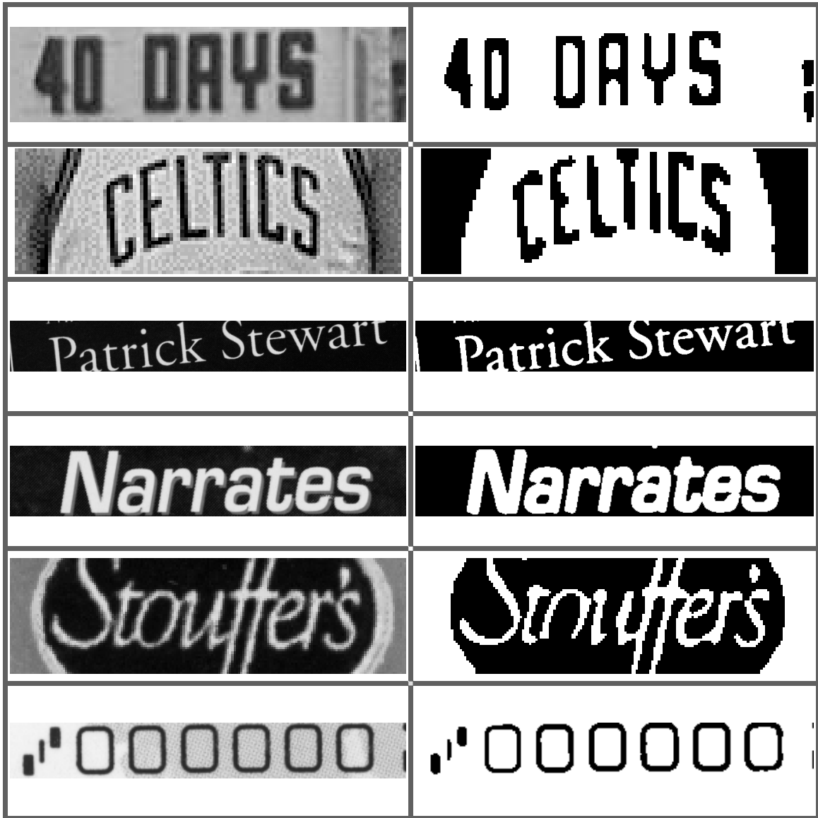
Figure 15: On the left are text chips generated by the text detectors; on the right are the corresponding results of the background removal algorithm.
