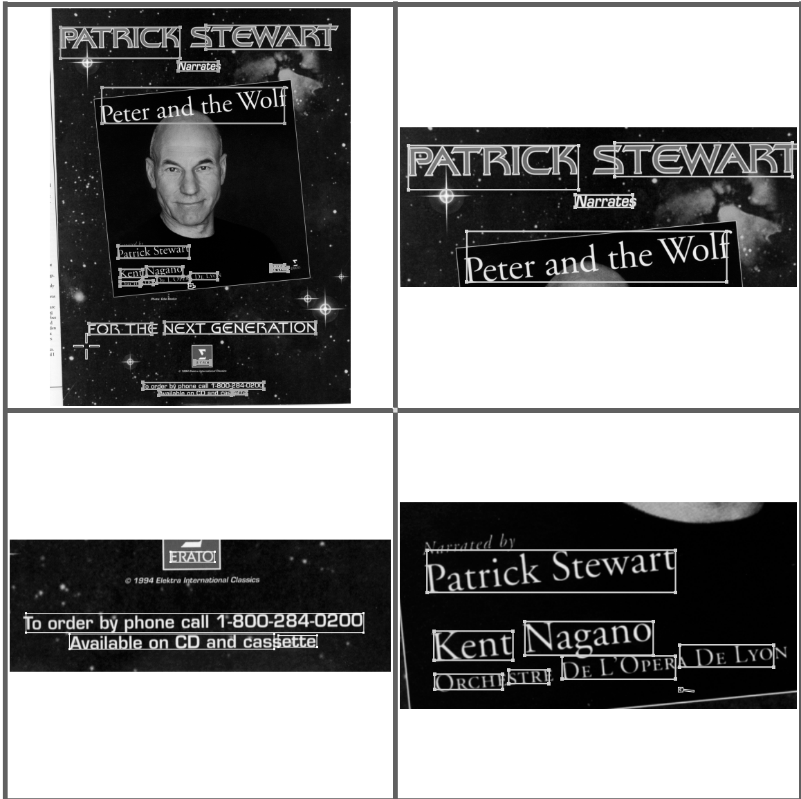
Figure 7: Upper left window shows the original image with rectangle boxes representing the identified text regions; the rest of the windows show magnified parts of the upper left window. The second text detector is used.
