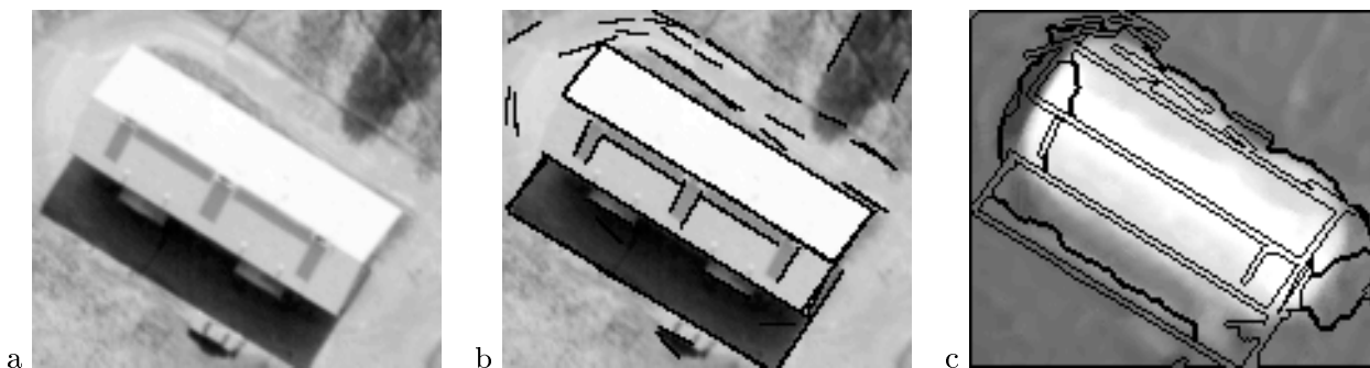
Figure 22: ISPRS peaked roof house (compare with Fig. 15b). (a) Optical image; (b) optical image overlaid with extracted lines; (c) brightened elevation map overlaid with boundaries of fitted regions (holes are not shown).
