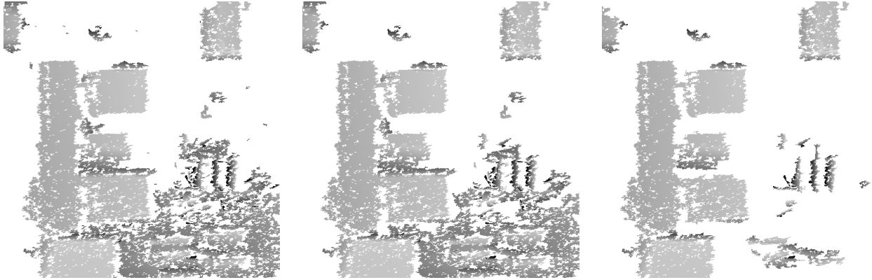
Figure 13: Same data as Fig. 11, but with ground regions removed with q = 1, 1.5, 2 (left to right). Lighter gray levels indicate higher elevation; white areas are not covered by any region. Note that q = 1.5 is the same value as used for the region generation (see text).
