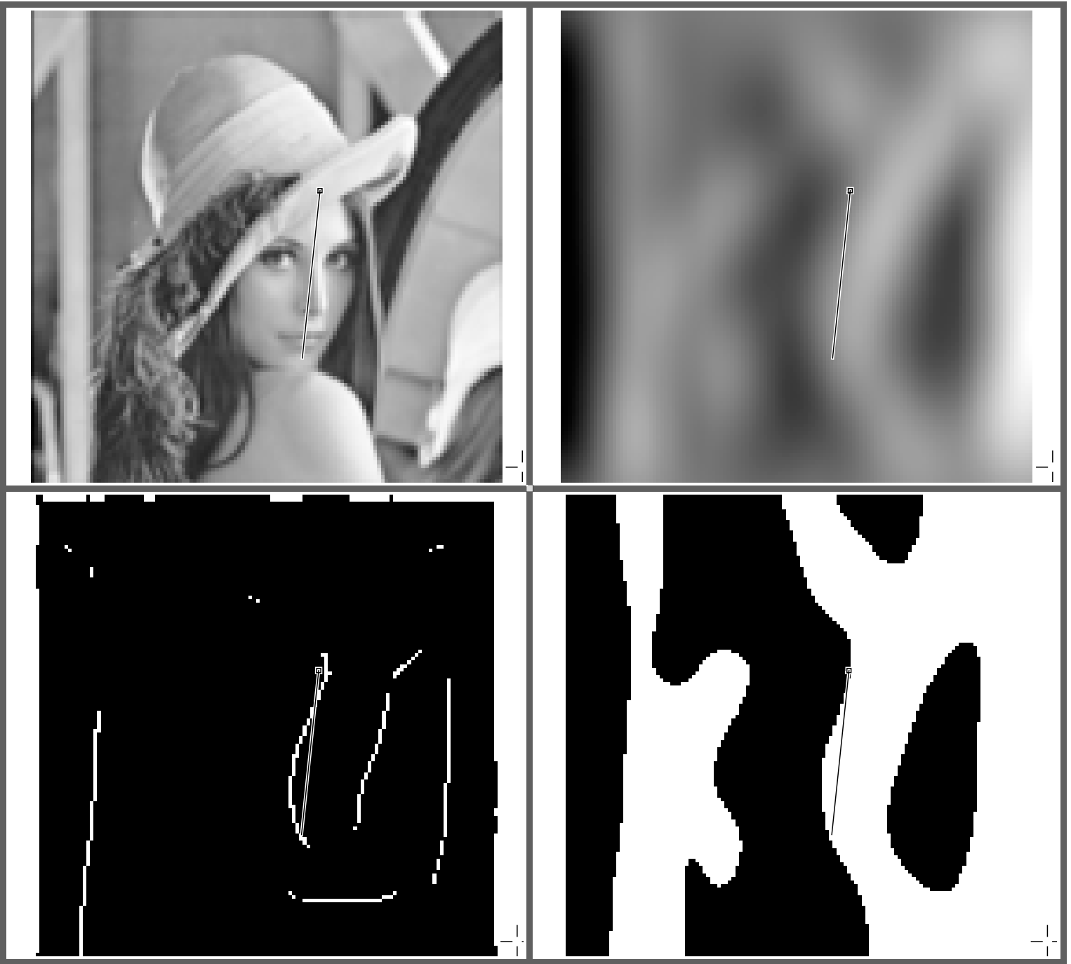
Top left: Lenna image 2 reduced. Top Right: d/dx image. Bottom left: the detected bilateral symmetry Bottom right: d/dx showing the zero crossings.
