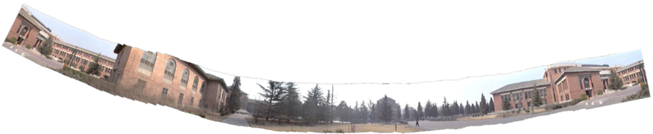
Fig 6(a). Unfolded conic mosaic (13% display scale). The original color image is 3806 x 773x24 bits. Notice the curved and uneven boundary created by the up-tilted angle and unstabilized motion of the hand-held camera.
