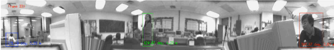
(1) 330c.tif: Current Cylindrical image, with bounding rectangles of moving objects superimposed
