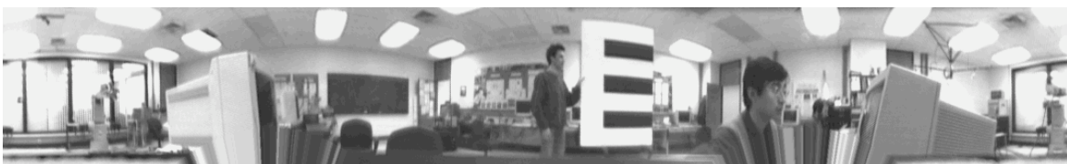
Fig. 4.3. Cylindrical panoramic image, after eliminating radial distortion
