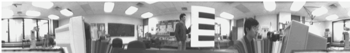
Fig. 2.4. Cylindrical panoramic image, after eliminating radial distortion
