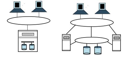
Figure 1: The server-attached disk architecture and network-attached disk architecture for file system design.
