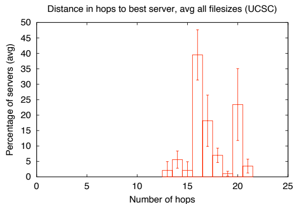
Figure 6: Distribution of distance in routers hops to the best server for UCSC.
