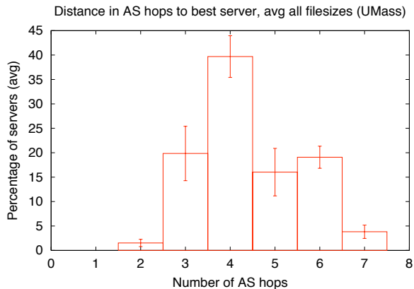
Figure 10: Distribution of the distance to best servers in AS hops for UMass, averaged for all file sizes and for all 193 servers.
