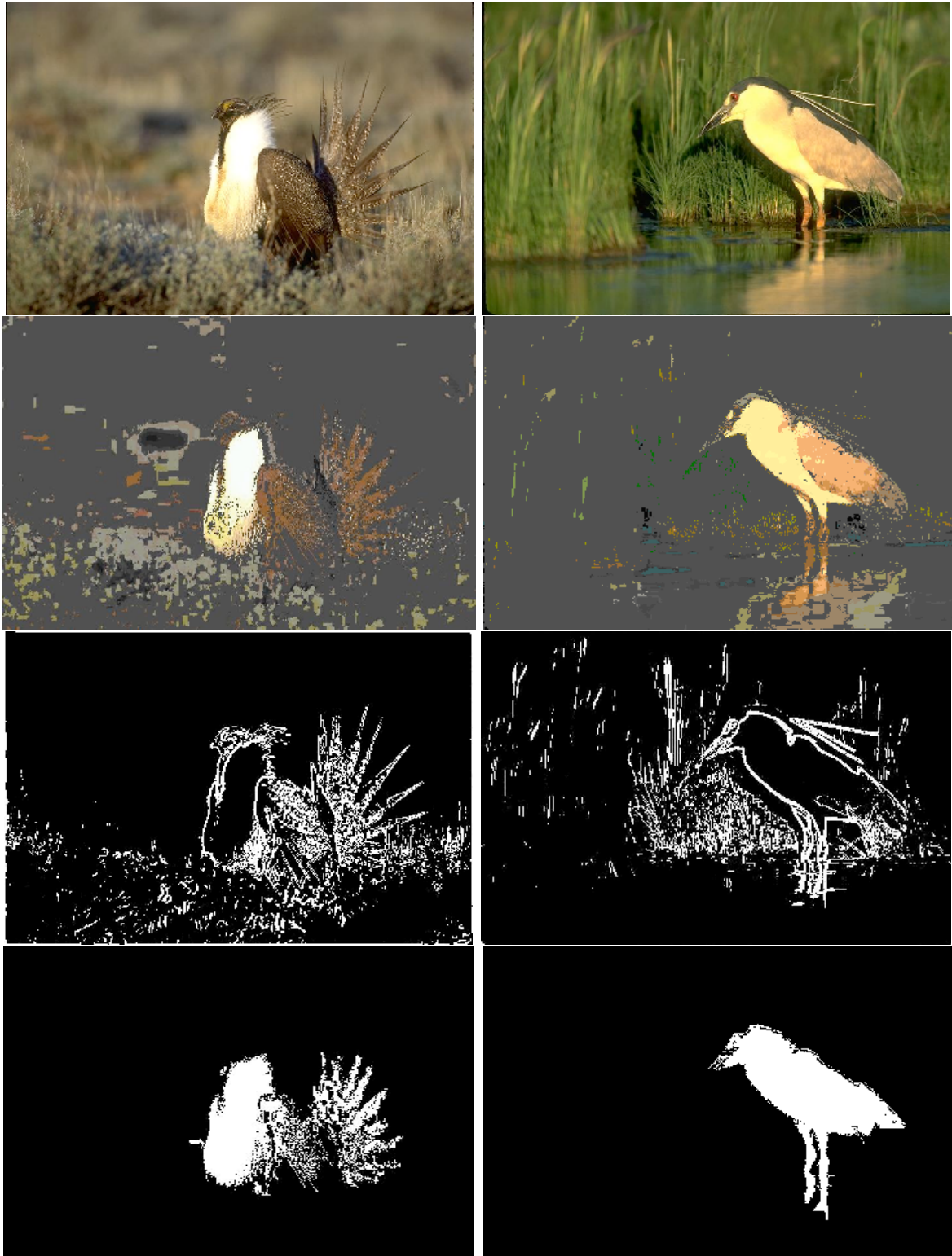
Figure 5.8. Examples of region of interest segmentation : (row 1) original images (row 2) remaining image after background colors are eliminated (row 3) edge image (row 4) final segment obtained
