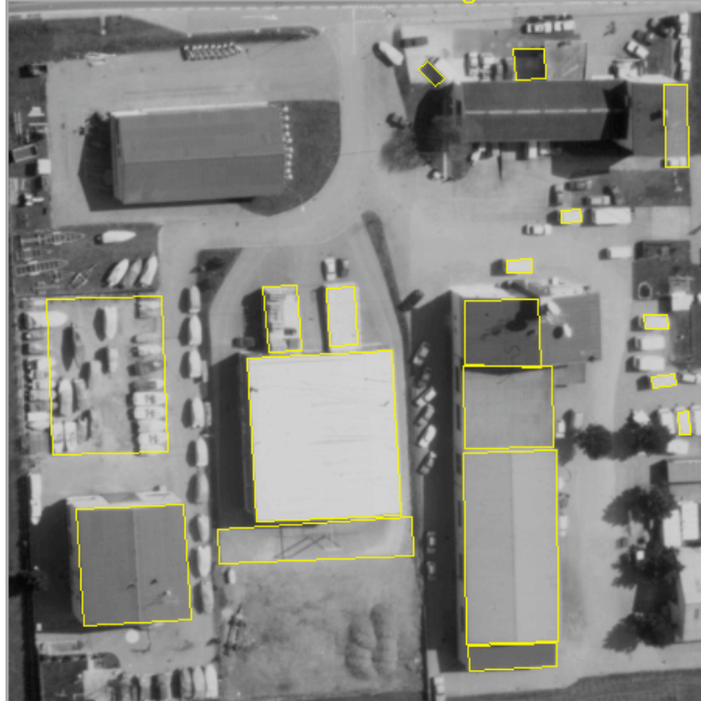
Figure 4.17. The input regions from the Avenches data set. These regions were obtained by running the original Ascender I system constrained to detect two-dimensional building footprints.
