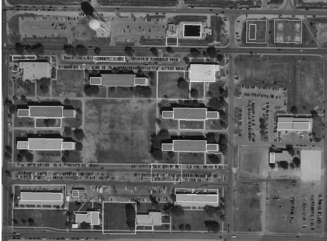
Figure 4.16. The input regions from the Fort Hood data set. These regions were obtained by running the original Ascender I system constrained to detect two-dimensional building footprints [16].
