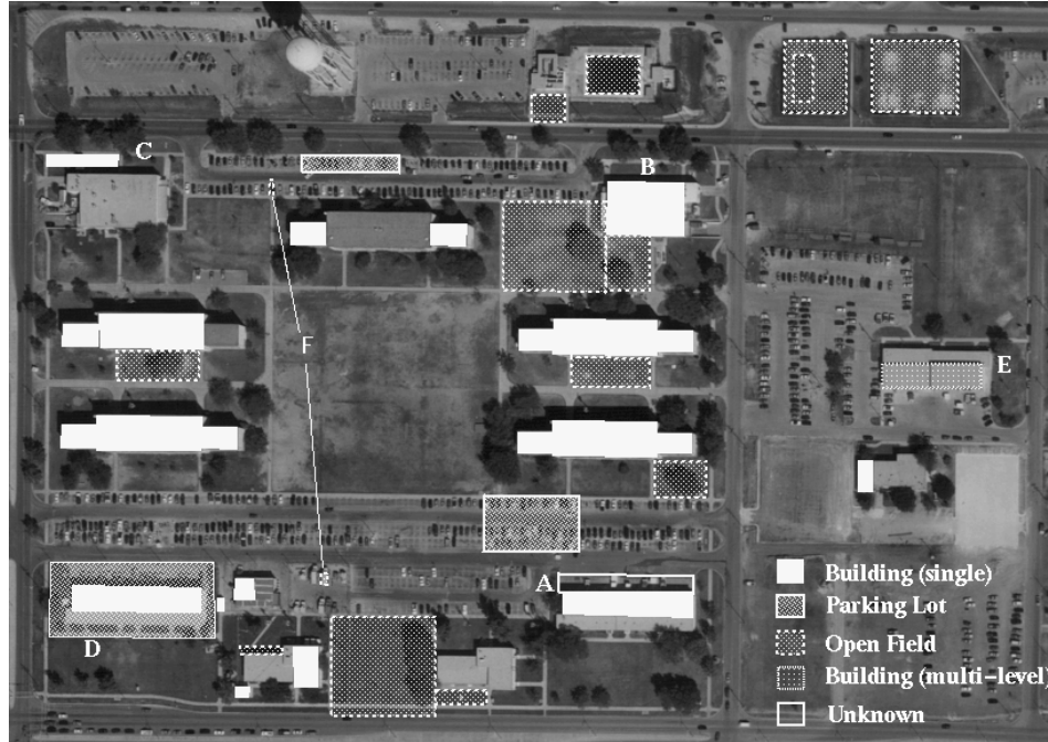
Figure 4.18. Recognition results on the Fort Hood data. Three regions were misclassified and for one region the system was not able to make a decision.
