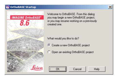
Select OK to create a new OrthoBASE Project. Navigate to the folder where you want to store your block file and type in a filename in the following window:
