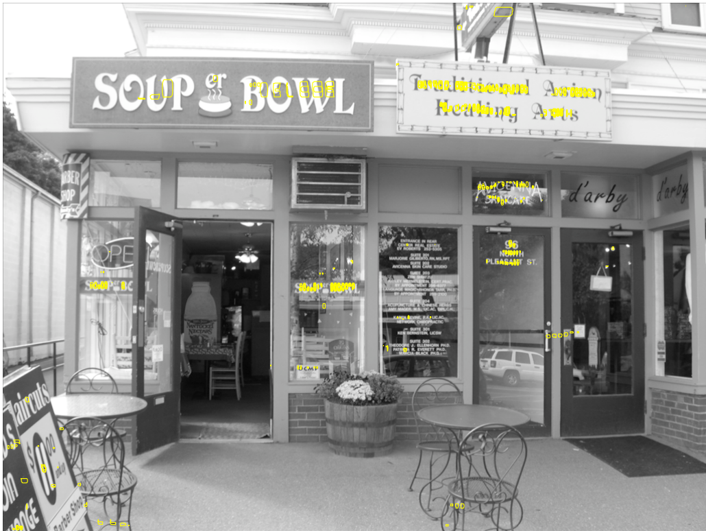
Figure 7: Text detection with grating cells (cf. Figure 1). TOP: Grating cell responses over several scales. BOTTOM: Contours of responses overlaid on the image.
