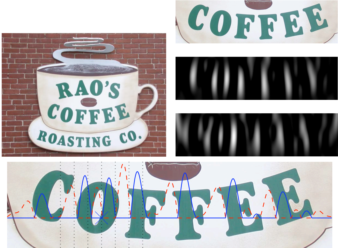
Figure 5: Grating operator on text. UPPER LEFT: Input image. UPPER RIGHT: Center-on and center-off simple filter responses ( \theta = 0 ). BOTTOM: Slice of simple filter responses (center-on in solid and center-off in dashed) with receptive regions for a marked point.
