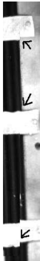
Figure 26: The arrows in this mosaic show misalignment at the top and bottom of the mosaic while there is alignment at the middle.
