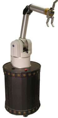
Figure 1: A platform for autonomous mobile-manipulation under construction at UMass
