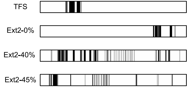
Figure 10: Block allocation pattern for several contribution levels in Ext2 and TFS. Both TFS and Ext2 with 0% contribution show high locality. The other systems do not because the contributed files interfere with the block allocation policy.
