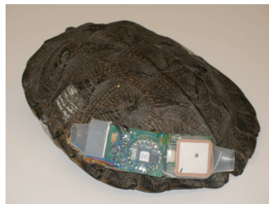
Figure 6: The energy measurement and charging board with a Mica2Dot, GPS receiver, and battery.
