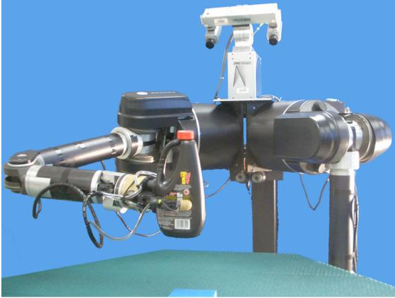
Fig. 1. This picture shows Dexter performing a grasp of the `black_drano` object, as described in Section VI. Each of Dexter’s arms has 7 DOF and is equipped with a three-fingered hand with four total degrees of freedom. The stereo head has four degrees of freedom.
