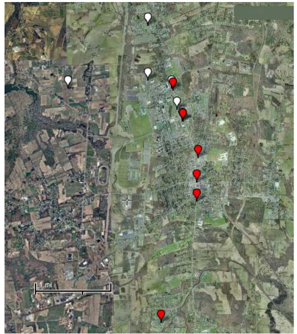
Figure 9: The map shows the location of the relay/mesh nodes and base stations. The colored spots represent the base stations and the white spots depict the relay/mesh nodes. For double blind reviewing, we removed the underlying map features.
