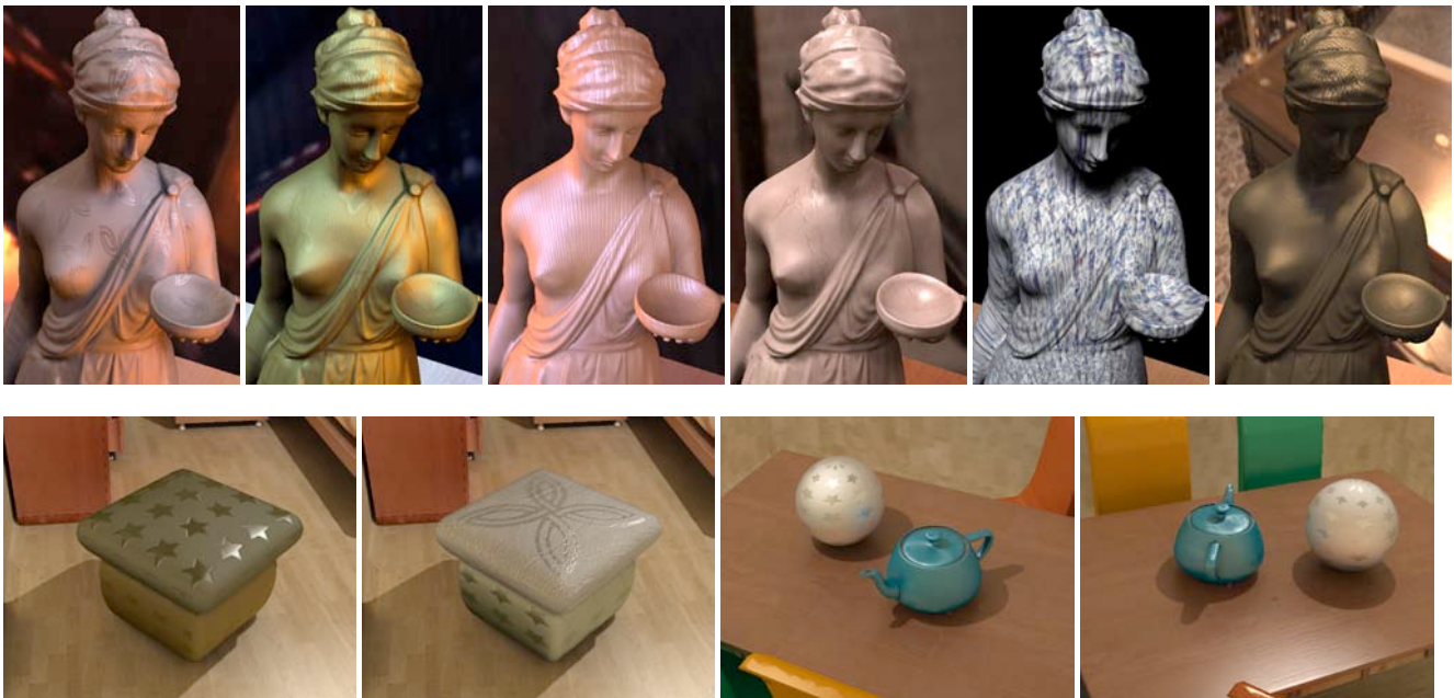
Figure 6: The upper row shows realistic material design on the model Hebe with changing environment lighting. Note the rich per-pixel shading effects. We use a combination of bump map and spatially-varying BRDF parameters. The first two images in the bottom row shows editing of the puff chair model with different materials; the right two images show ward anisotropic BRDF applied on the teapot and a star specular map applied on the sphere.
