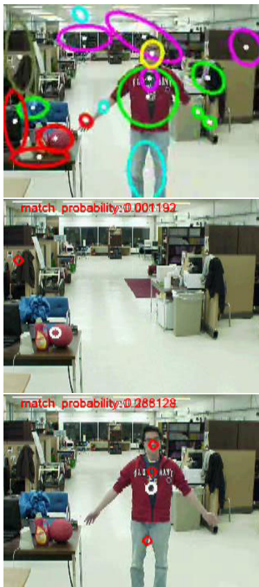
Figure 5: Human detection test. (a) Features extracted in a natural scene with cluttered background, (b) current most probable location (white circle) of a human, though probability is low (0.01192), (c) with presence of a human, a proper estimate is made with a higher confidence(0.288129).
