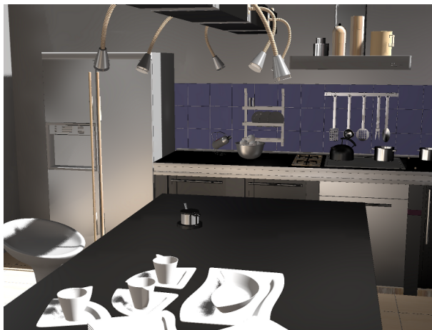
Figure 1: A screenshot captured at 7 fps with 768 \times 512 res., glossy materials, 2 bounces of indirect lighting, and 2 \times 2 supersampling.
