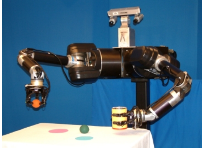
Figure 3.2. The bimanual robot “Dexter.”
