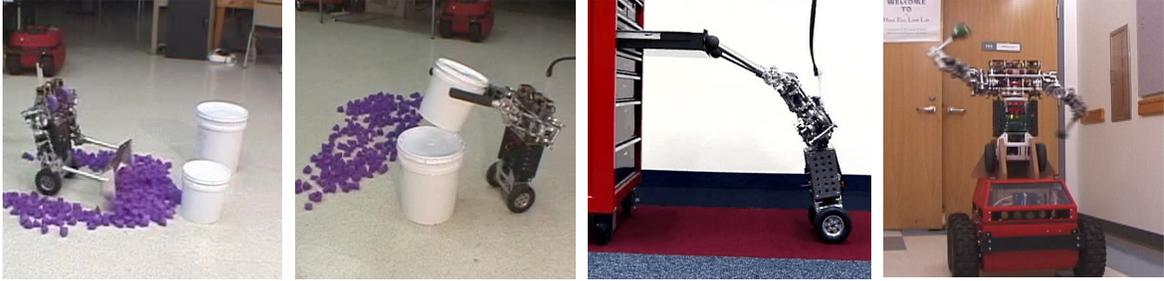
**Figure 6.5.** The uBot performing plowing, stacking, pushing, and throwing tasks.
