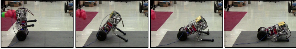
Figure 3: Bracing policy execution after a large impact perturbation. Total duration of the above sequence is 0.7 seconds.
